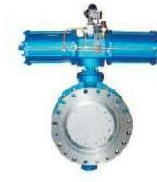
Flanged Multi-Layer Metallic Hard Swirling Butterfly Valve (GB, ANSI, JIS, DIN, BS) (CF8, CF8M, WCB) DN50~600 / 2"~24" PN16~63 / 150LB~300LB / 10K~20K
