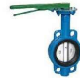
Hand Operated Wafer Type Rubber Lined Butterfly Valve (GB, ANSI, JIS, DIN, BS) (CF8, CF8M, WCB) DN50~600 / 2"~24" PN16~63 / 150LB~300LB / 10K~20K
