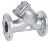
ANSI, JIS, D.N., CB Flanged Strainers (CF8, CF8M, WCB) ANSI-1/2"~20" / 150LB~300LB JIS-DN15~700 / 10K~20K DIN-DN15~700 / PN16~40 GB-DN15~7500 / PN16~40
