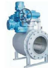
Flanged Ball Valve With Electric Actuator (CF8, CF8M, WCB, TI, NI) ANSI- 2"-28" / 150LB-300LB JIS- DN50-700 / 10K-20K DIN, BS- DN50-700 / PN16-63 GB- DN50-700 / PN16-63
