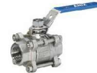
3PC Type Ball Valve With Internal Thread (CF8, CF8M) 1/4"-4" / 1000PSI
