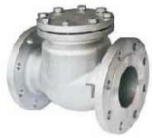
ANSI, JIS, DIN, GB Flanged Check Valve (CF8, CF8M, WCB) ANSI-1/2"~24" / 150LB~300LB JIS-DN15~500 / 10K~20K DIN-DN15~500 / PN15~63 GB-DN15~500 / PN16~63
