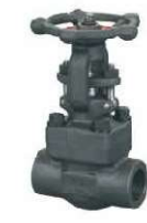
ANSI Standard Forged Steel Gate Valve (A105, F304, F316) 1/2"~24" / 150LB~900LB
